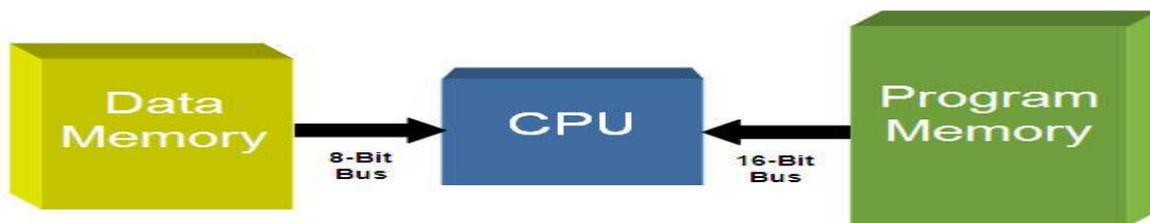
Fig. 4: Simple Block Diagram Of CPU Interfacing With Data And Program Memory In PIC
